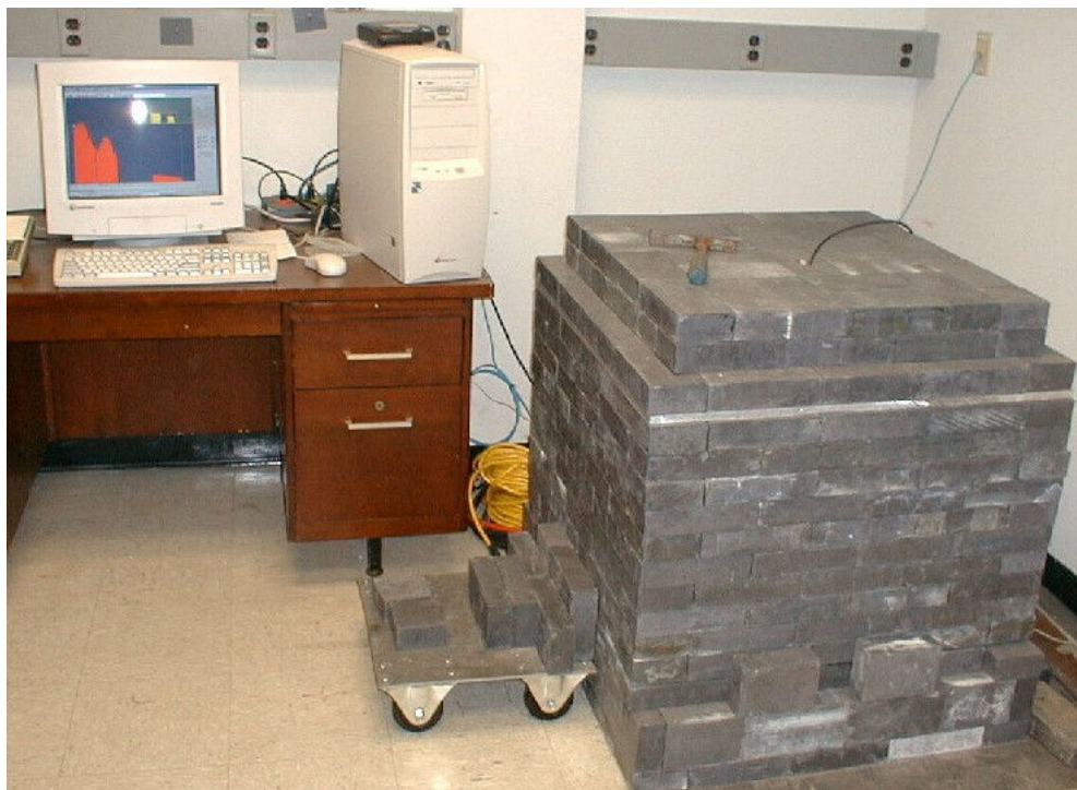
Fig. 4.63.2: ^{152}\text{Eu} is used as a reference source for calibrating gamma-ray spectrometer systems like the one pictured here. (Photo Source: Snyder and Duval, 2003. U.S. Geological Survey Open-File Report 03-029) [447].
