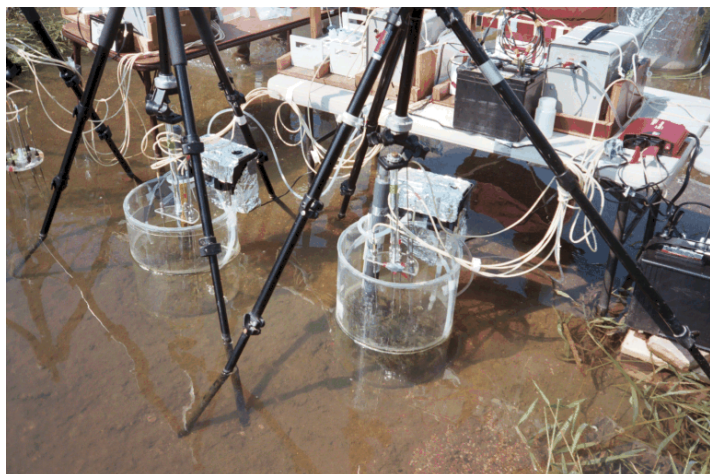
Fig. 4.7.2: Tracer experiments with the stable isotope ^{15}\text{N} have been used to track excess dissolved nitrate in groundwater and streams and to determine to what extent the dissolved nitrate is removed by natural processes, such as conversion to harmless \text{N}_2 gas before entering nitrogen-sensitive ecosystems [80]. (Photo Source: Böhlke, J.K., U.S. Geological Survey).
