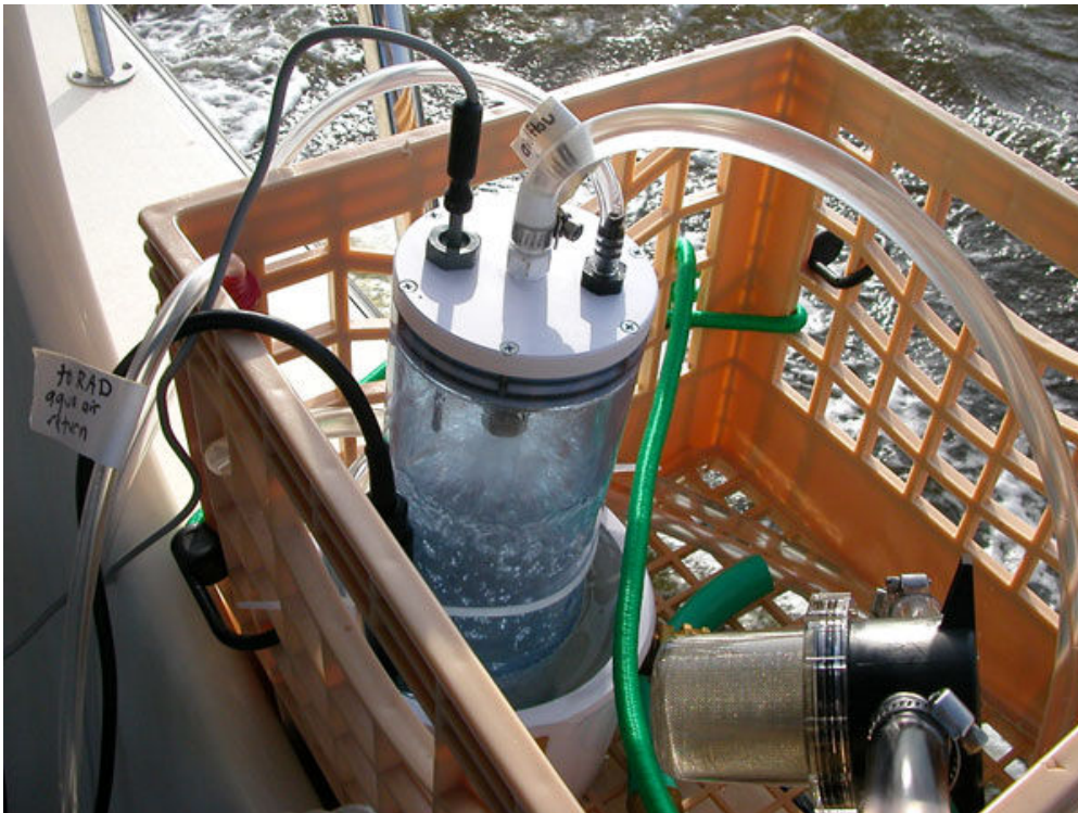
Fig. 4.86.1: Air-water equilibrator, which strips radon out of water and into the gas phase so it can be used as a groundwater tracer . (Photo Source: John Crusius, U.S. Geological Survey) [570].
